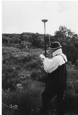
Figure 14. RTKGPS roving unit
