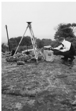
Figure 13. RTKGPS base station
